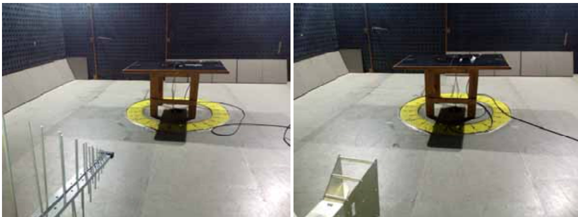
Photograph 7.2.2 Setup for final radiated emission measurements, EUT cabling, CR300B 2G NA, part number CT7801201-000
