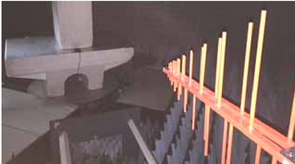
Photograph 7.1.2 Setup for radiated emission measurements, EUT cabling, CR300B 3G NA, part number CT7801200-000
